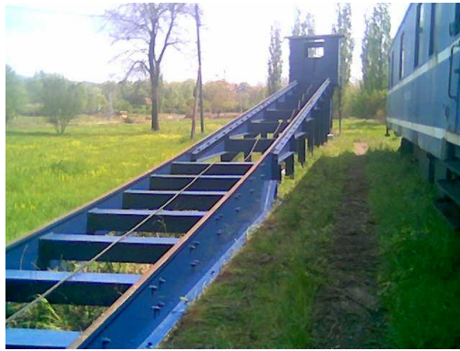
Fig. 5. Rig for impact tests of wagons in Kraljevo
