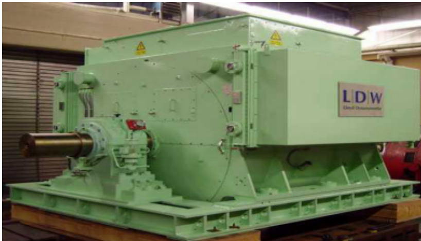
Sinhroni generator snage 15 MVA
