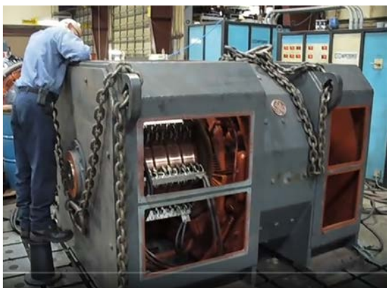
Сл. 28 2000 hp (1,47 MW) DC motor
