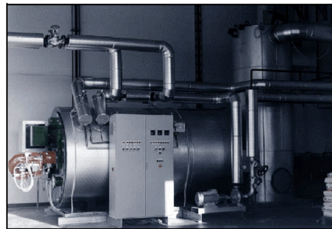
Figure 4.27: Unit for direct-flame incineration with afterburner [65, Germany, 2002]
